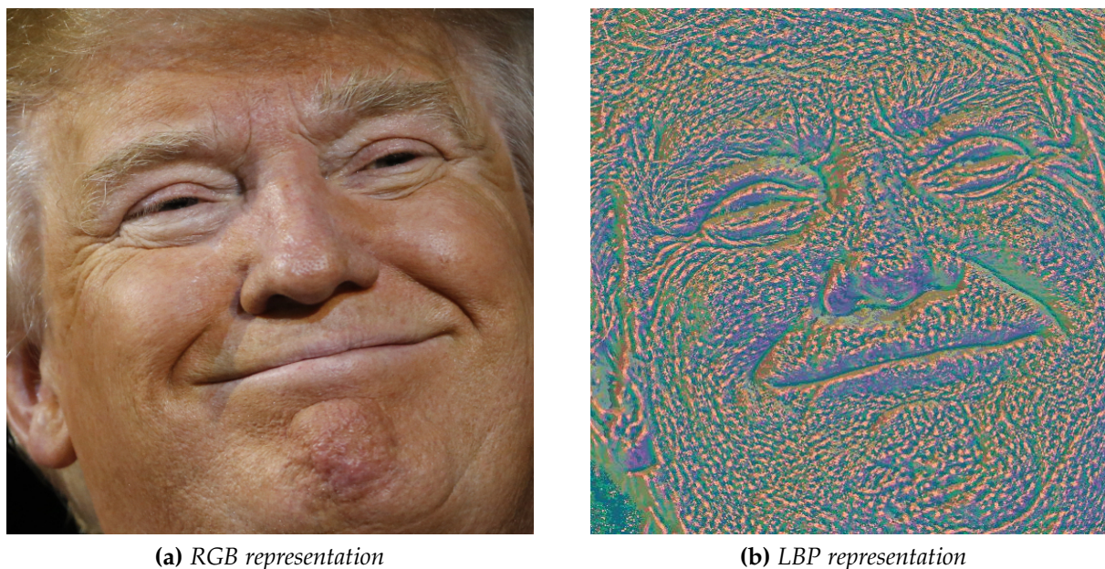
Figure 1: On the left, an example image in its RGB (red, green and blue) representation. On the right, the same image in its LBP (Local Binary Pattern) representation. This is the input to the neural network and provides better accuracy than its RGB counterpart.
